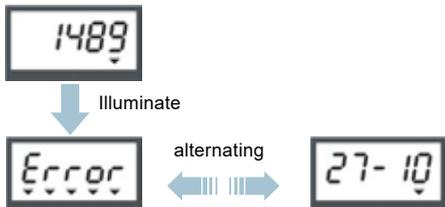
If a device failure is present, in all display menus a black triangle is being shown under the last digit.
