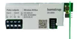
The wireless M-Bus module must be connected to an internal or external antenna. When mounting an external antenna, ensure that the antenna cable is not jammed or damaged when the calculator is assembled. Before replacing or mounting modules, the supply to the meter must be switched off. The same applies to mounting of an antenna.
