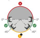
The flow sensor can be mounted at an angle of 0° and may be turned 90° downwards.
