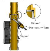
Kamstrup flow sensors require neither straight inlet nor straight outlet to meet the Measuring Instruments Directive (MID) 2014/32/EU, OIML R75:2002 and EN 1434:2015. A straight inlet section will only be necessary in case of heavy flow disturbances before the meter. It is recommended to follow the guidelines of CEN CR 13582.
