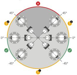
The flow sensor can be mounted at an angle of 0° and may be turned 45° upwards or 90° downwards.
