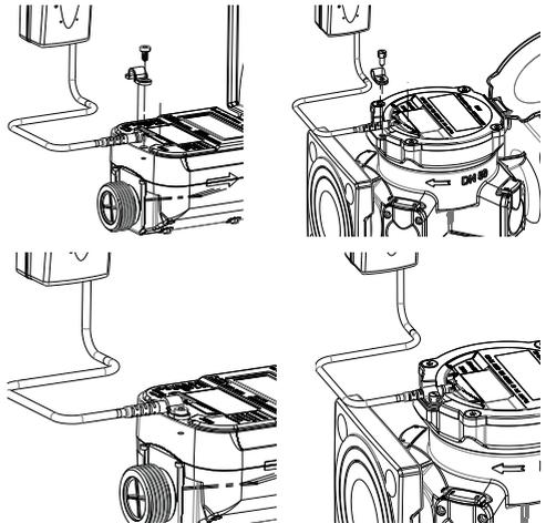
4. Fasten the NDC LoRa / wM-Bus module to the desired installation point – depending on local conditions – either using the existing wall mounting or cable ties. Attach the three respective ten metre long connection cable in such a way that a risk of injury is not posed.
