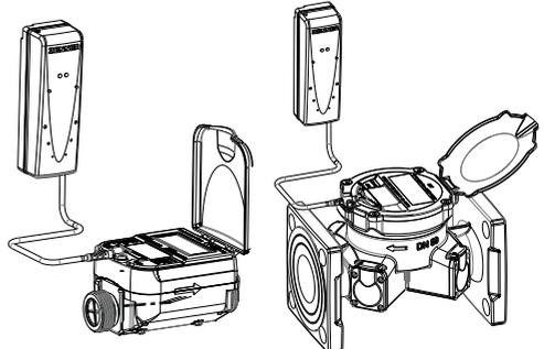
5. Where possible, ensure that no metallic objects impede the radio emission of the NDC module.
