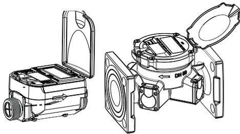
2. Release the standard ex works NDC dummy module from the water meter which is used to protect the NFC interface of the meter. For this purpose, loosen the fastening screw with the appropriate screwdriver and remove the plastic dummy.
