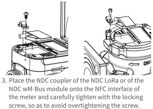
3. Place the NDC coupler of the NDC LoRa or of the NDC wM-Bus module onto the NFC interface of the meter and carefully tighten with the locking screw, so as to avoid overtightening the screw.
